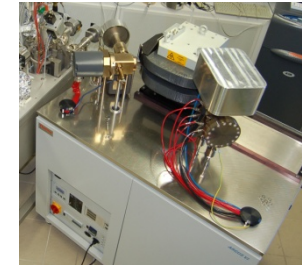
An ARGUS VI noble-gas mass spectrometer
