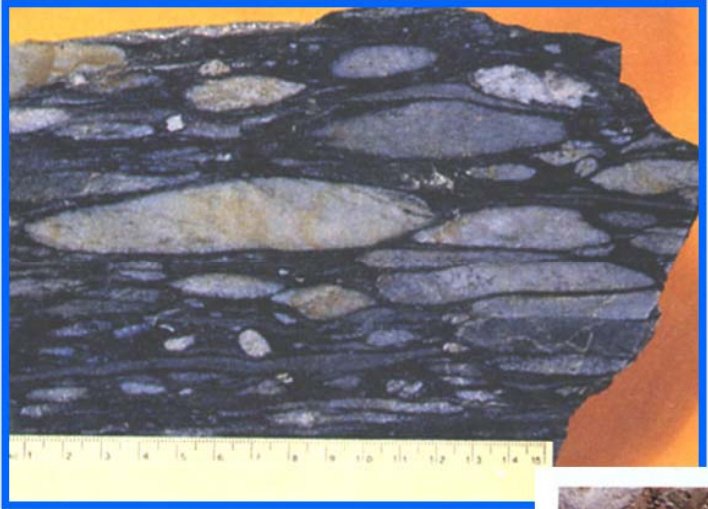
Conglomerate cobbles that have been flattened (left) compared to an unstrained conglomerate (below).
